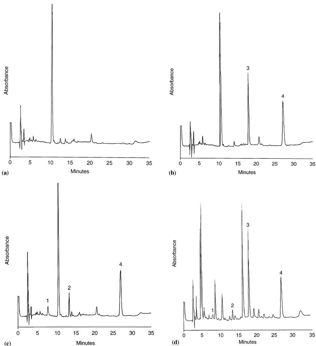
Fig. 3. Representative chromatograms of: (a) drug free human serum; (b) spiked serum containing  $10 \mu\text{g ml}^{-1}$  vancomycin; (c) spiked serum containing  $2.5 \mu\text{g ml}^{-1}$  CDP-1; and (d) a patient's serum containing  $12.0 \mu\text{g ml}^{-1}$  vancomycin and  $2.5 \mu\text{g ml}^{-1}$  CDP-1. Peaks: 1, CDP-1-m; 2, CDP-1-M; 3, vancomycin; 4, cefazolin (internal standard).
